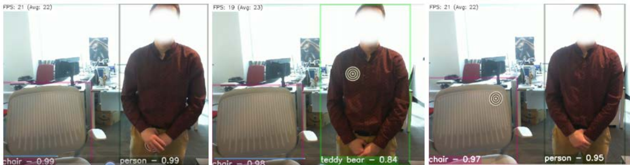
Figure 5. [Left] example output of an object classifier on one frame of video data. [Centre] the result after placing the trigger on a person. [Right] the result after placing a trigger on a different object.
